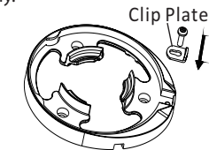
Figure 2-2 Screw the Clip Plate
